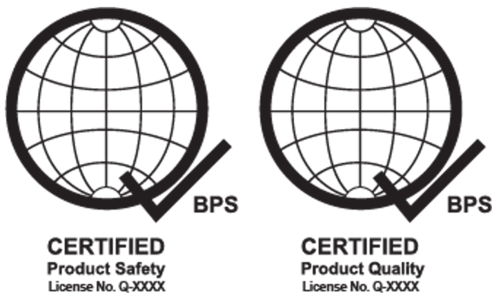
Figure 2: Marking in a RAC Appliance issued by DTI-BPS through a Product Certification Scheme
